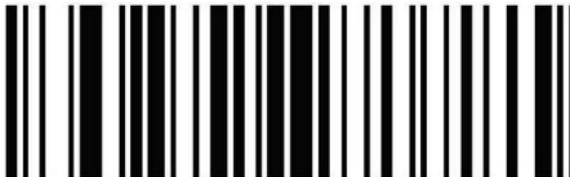
After scan "Add Enter" barcode, it can automatically move to next line in the text field after each scanning. If user wants to close the function, scan "Delete Enter" barcode.
